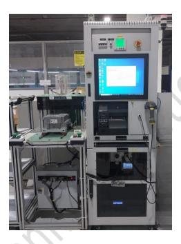
The ATE system incorporates specialized test interfaces, test fixtures, and test programs to facilitate comprehensive testing of motor control units. These components allow for precise control and monitoring of the motor control signals and responses.
